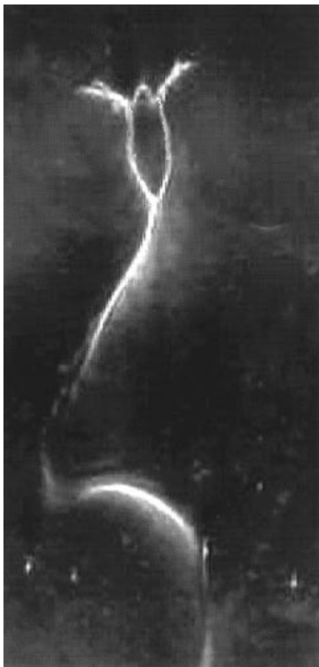
Figure 7. Photograph of hydromechanical trail ( 20\times ) created by a female Daphnia swimming through water. Trail is visualized by using a Schlieren optical path and a smooth density gradient as in Strickler (1977).
